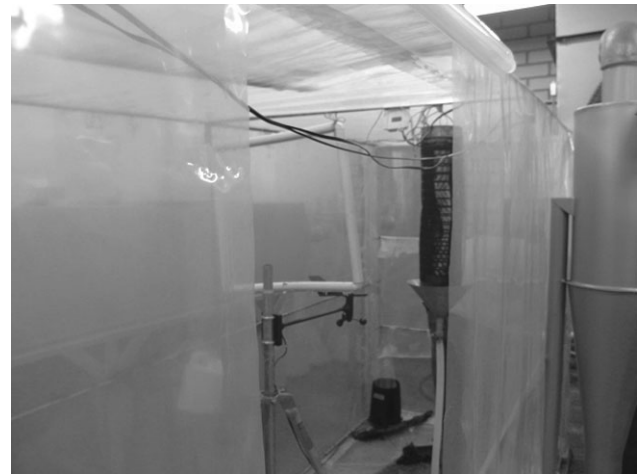
Figure 2. The fog chamber, a controlled volume containing two types of fog gauge: polypropylene harp (unidirectional gauge; left) and a Juvik cylinder (multidirectional gauge; right), where 21 fog events were simulated
